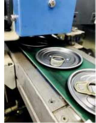
Ends with a randomized direction of the tabs leave the Randomizer.
