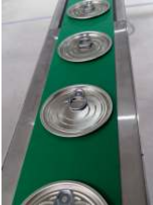
Ends with tabs in the same direction enter the Randomizer.
